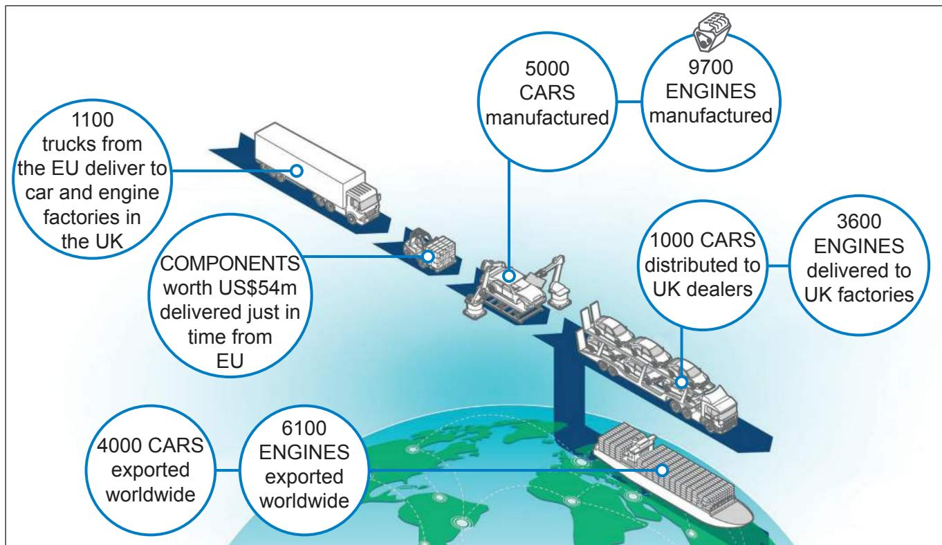
The manufacturing system shown is known as just-in-time where parts are ordered and received as they are needed, with minimal storage of parts at the factory.
